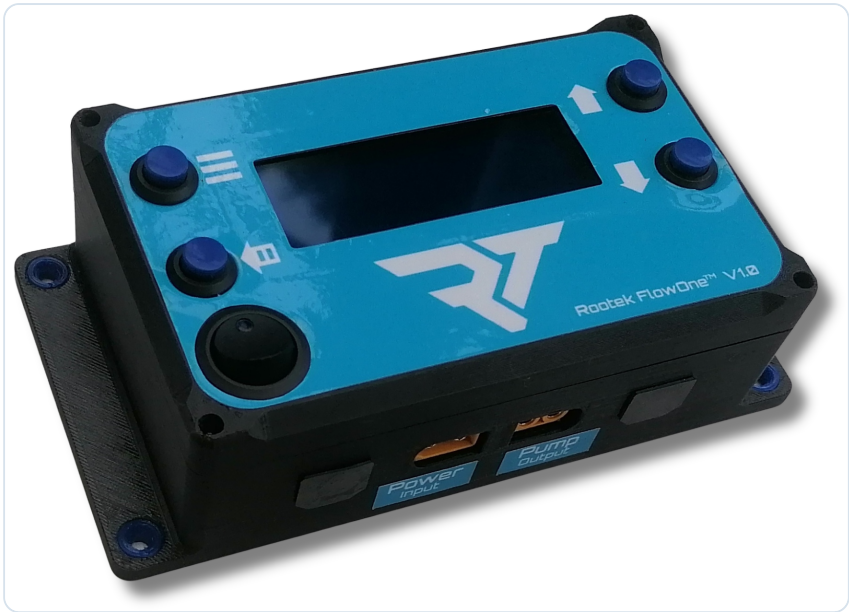
Menu (≡) and Back (◀) on the left, Up and Down on the right, power switch bottom left.
